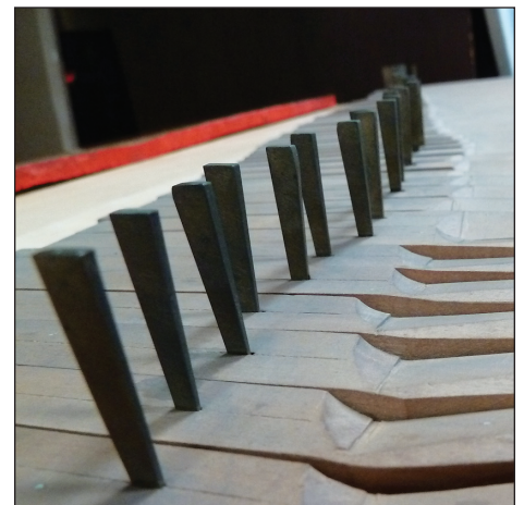
The tangents in the Bass section of Berlin 914, also showing the scribelines and the typical carving pattern found on all existing JHS clavichords with the exception of the instrument in Vienna
