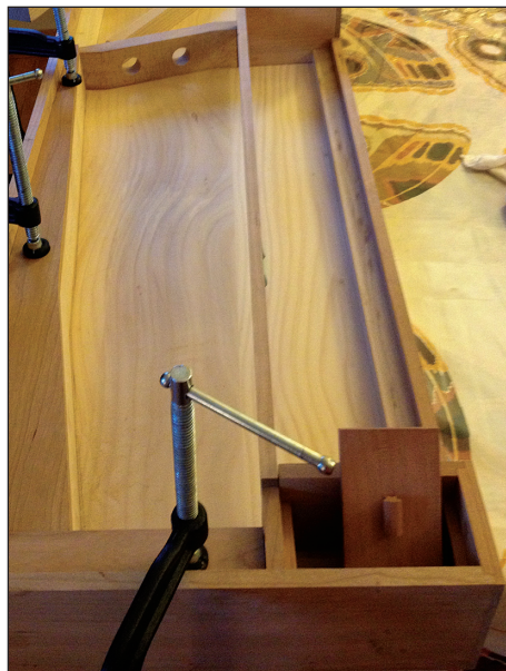
Clamping the hitchpin block and hitchpin dogleg
