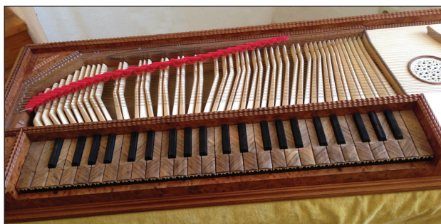
Clavichord by Andreas Hermert, 2009, after an anonymous clavichord of about 1700 in the Berlin Musical Instrument Museum, No. 2160, C/D-c", double fretted, played in Berlin
