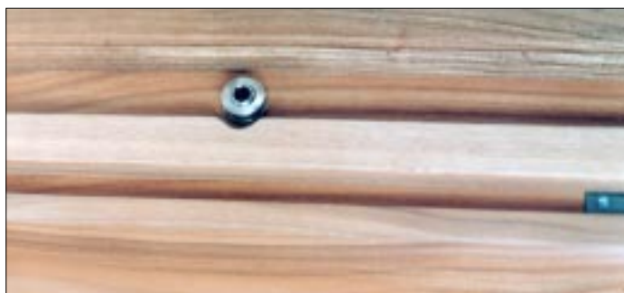
Photo 3 “The pin jack of the pick-up is placed at the back of the instrument through the case.”
